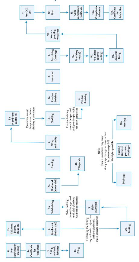
Any of the above inspections may occur more than once, for example there maybe multiple inspections of any type. When there is a slab plumbing, this should occur before slab building, similarly when there is a pre-line plumbing this should occur before the pre-line building it is also possible for some inspections to occur at the same time.
