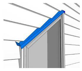
Raked window head flashing – fully welded
