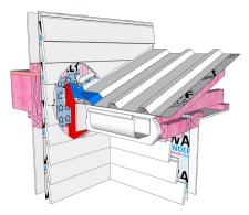
**Step 4:** Finished cladding and gutter/fascia board termination in relation to cladding
