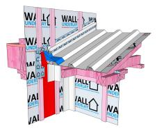
**Step 3:** Overlap wall underlay from above, flashing tape and cavity battens
