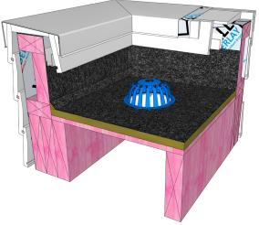
Proprietary outlet with membrane clamped by screw fixed grate or dome
