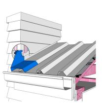
Gutter/fascia junction at parapet corner
