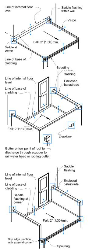
Membrane decks, roofs and gutters have a high occurrence of weathertightness failure. Often this can be due to surfaces having been constructed with minimal falls, tiles having been fixed directly to the membrane, and perimeter junctions and walls lacking adequate flashing. Membranes have also failed due to movement in substrates, age and/or poor maintenance.
