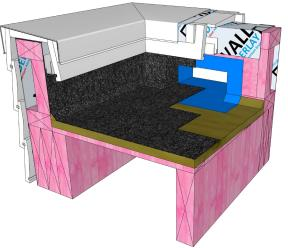
Membrane applied into preformed scupper
