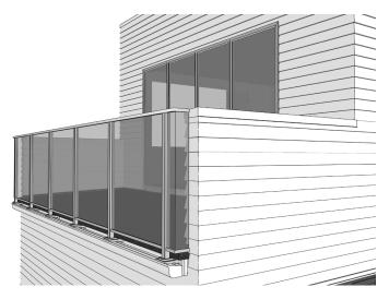
structurally fixed. In these instances, the balustrade manufacturer will generally recommend that an engineer be engaged to verify the structure supporting the balustrade is of sufficient capacity to resist balustrade applied loads.
