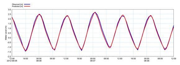
Figure 4-4 Comparison of observed and predicted water levels at Helensville tide gauge for June 2012 validation event
