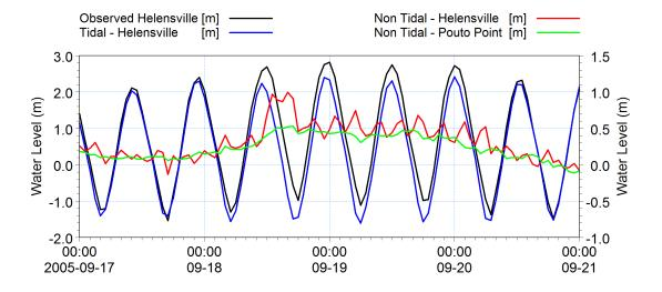
Figure 4-1 Tidal analysis of observed data from the Helensville and Pouto Point Tide gauges for 2005 calibration event. Observed Helensville water levels and tidal component of Helensville water levels (left y-axis) and non-tidal component of Helensville and Pouto Point water levels (right y-axis)
