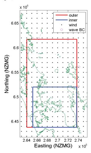
Figure 4-5: Outer and inner SWAN wave model grids of the Hauraki Gulf.
