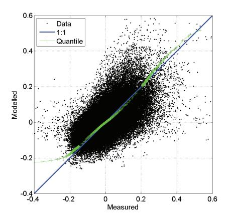
Figure 4-3: Scatter plot of measured (tide gauge) and modelled (WASP) storm surge at Port of Auckland (Waitemata), with quantile-quantile comparison.
