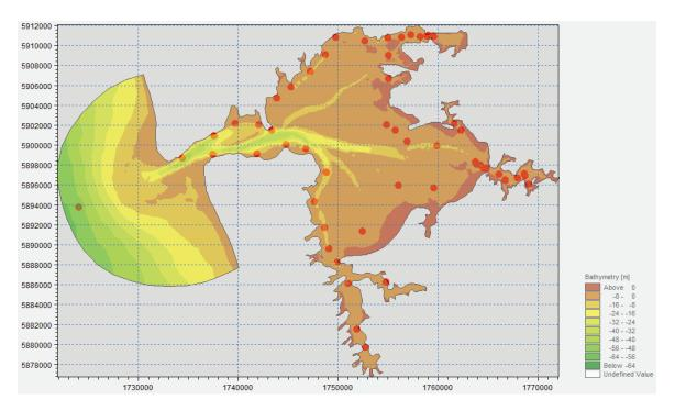
Figure 3-12: Hydrodynamic model bathymetry, with output locations marked.
