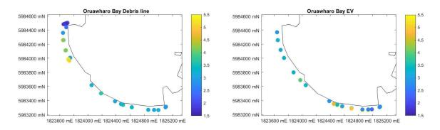
Figure 2-6: Intra-bay variation in beach feature elevation at Oruawharo Bay; Debris lines (left) and edge of vegetation or EV (right). NZ coast outline (black). Coloured points show surveyed elevation in m AVD-46. [Coordinate system: NZ Transverse Mercator 2000].
