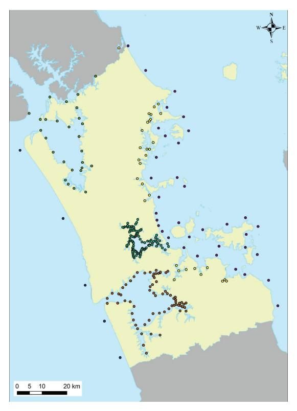
Figure 8-1: Map of the Auckland Region with 0.01 AEP storm-tide elevations marked at model-output locations.
