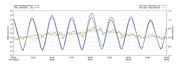
Figure 4-3 Tidal analysis of Helensville and Pouto Point Tide gauges for validation event. Observed Helensville water levels and tidal component of Helensville water levels (left y-axis) and non-tidal component of Helensville and Pouto Point water levels (right y-axis)
