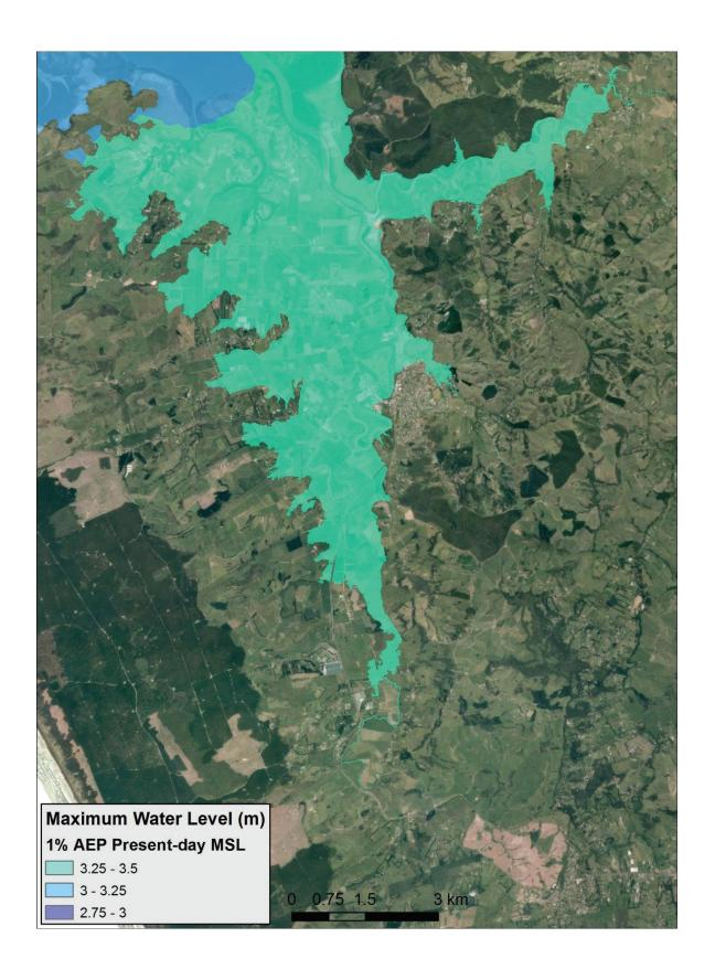
Figure 2-6: 1% AEP coastal-storm inundation elevations at present-day MSL mapped by NIWA in 2013.
