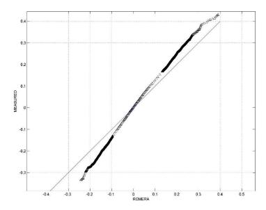
Figure 4-16: Quantile-quantile comparison of storm surge derived from the Anawhata tide gauge and the WASP model. (RCMERA = WASP model; Measured = Anawhata tide gauge.)
