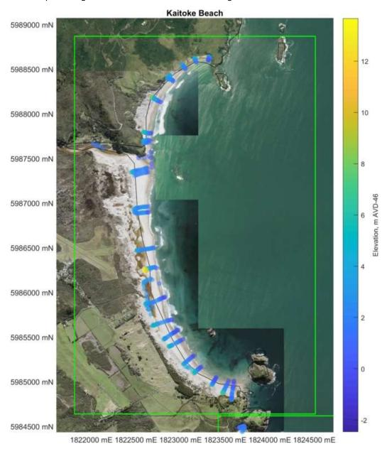
Figure 2-2: Example survey point distribution at Kaitoke Beach showing cross-shore beach profiles and elevation of survey points. Figure includes all survey points and does not delineate between beach features. [Aerial photograph: Auckland Council GIS, Coordinate system: NZ Transverse Mercator 2000].
