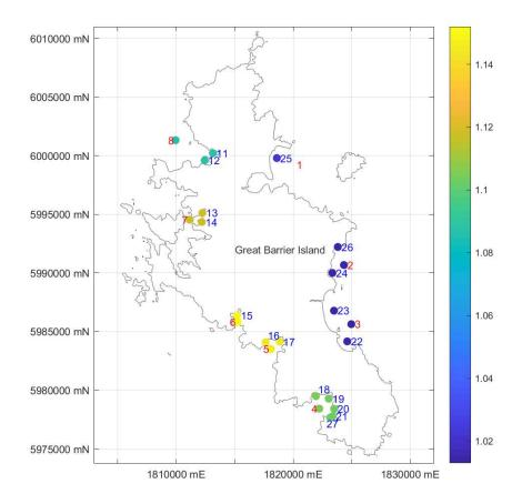
Figure 2-12: Spatial distribution of MHWS10 elevations around Great Barrier Island. Colour represents elevation relative to MSL - to make them relative to AVD-46 requires the addition of MSL datum offset (+0.15 m). Refer to Table A-1 for site coordinates and site name/number reference. [Coordinate system: NZTM].
