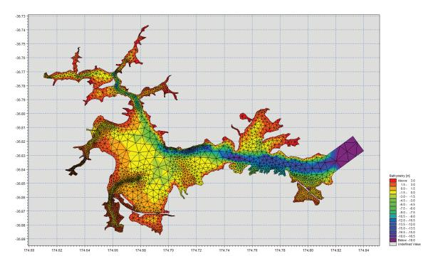
Figure 3-5: Waitemata Harbour MIKE-3 FM hydrodynamic model grid (Oldman et al. 2007). (Note: idealised channel created for eastern boundary condition)
