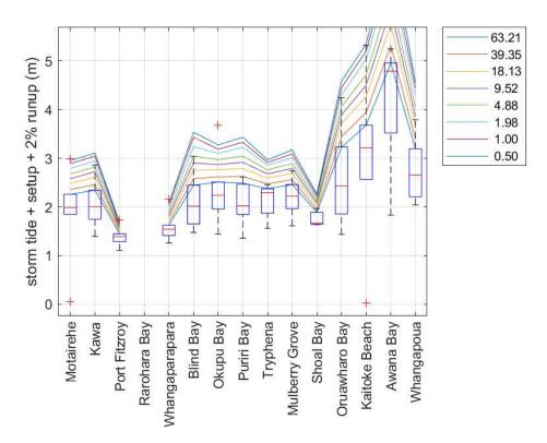
Figure 2-21: Return values of the vertical level of storm tide plus wave runup and setup, with beach slope tuned to match the 63% AEP value against the 75th percentile value of debris line elevation. Corresponding AEP values for total water level are shown in the legend. Box plots show the minimum, maximum, 25th, 50th and 75th percentile values of debris line elevation.
