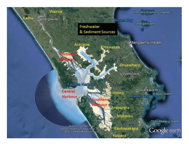
Figure 3-17: Aerial photo of the Kaipara Harbour and tidal inlet with Delft3d model grid overlaid.
