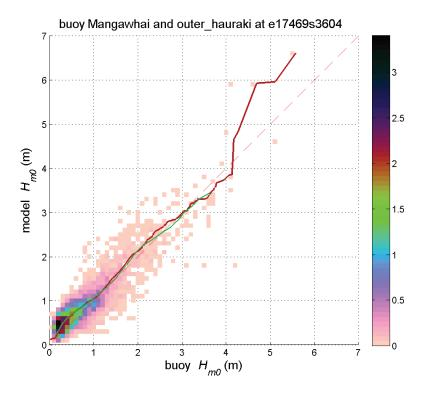
Figure 4-9: Comparison of significant wave height (Hm0) values predicted by the outer Hauraki Gulf SWAN model with measurements from the Mangawhai wave buoy.
