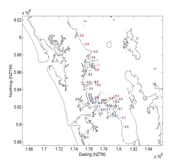
Figure 4-14: Difference between 1% annual exceedance probability storm-tide plus wave setup and storm-tide-only elevations on the eastern open-coast.
