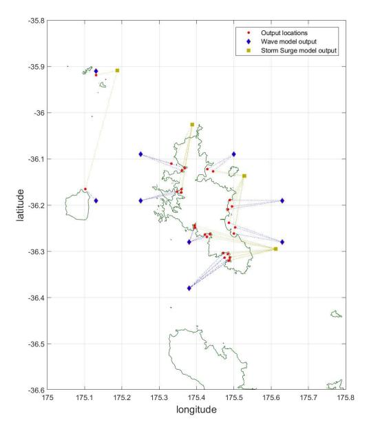
**Figure 2-15:** Map showing locations from which WASP hindcast outputs were extracted for each nearshore **location.** Sheltering and scaling corrections were applied to wave model outputs (from locations marked by triangles), while scaling corrections were applied to storm surge outputs (from locations marked by squares) to derive nearshore conditions (locations marked by red dots). Dotted lines connect nearshore locations with the relevant offshore model output locations.
