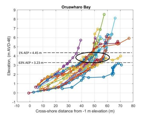
Figure 2-24: Cross-shore transects (coloured lines) measured at Oruawharo Bay with predicted 1% AEP and 63% AEP (annotations, dashed lines) extreme storm-tide + wave runup (including setup) elevations, and identified "slope break" zone (black oval). Horizontal axis is the linear cross-shore distance from the profile interpolated to the -1 m elevation. Elevations in m AVD-46.
