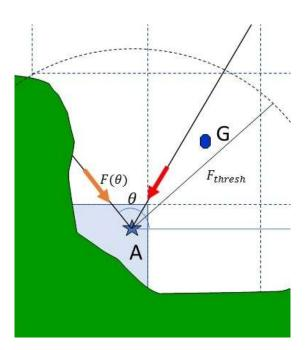
Figure B-1: Illustration of the sheltering correction method. Adjustments are applied to wave statistics extracted from a hindcast grid cell (G) to represent conditions at a nearshore point (A) to account for the direction-dependent fetch  $F(\theta)$  to the coast (the green area represents land).
