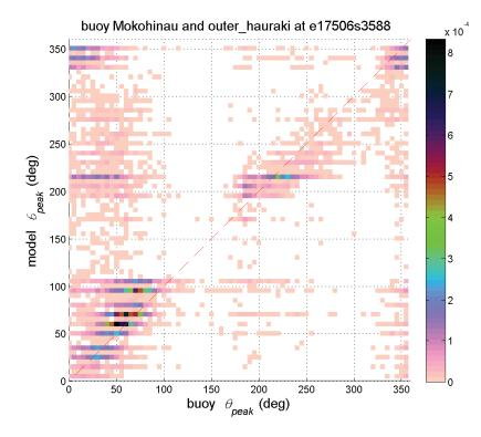
Figure 4-8: Comparison of peak wave direction (θpeak) values predicted by the outer Hauraki Gulf SWAN model with measurements from the Mokohinau Islands Waverider buoy.
