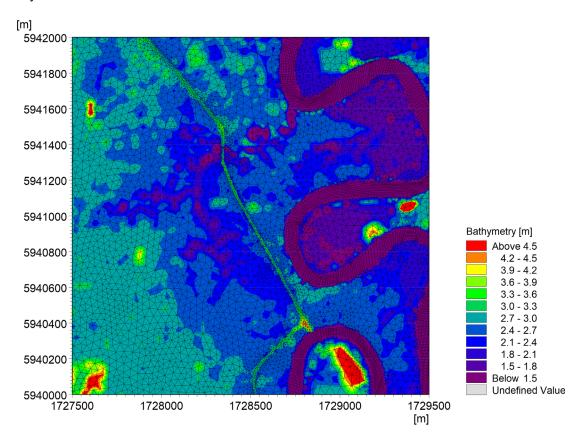
Figure 3-2 Parkhurst Road representation in model mesh. Depths are shown relative to Auckland vertical datum (1946).
