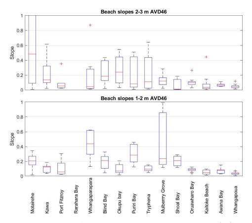
Figure 2-10: Bay by bay overview of measured beach slopes around Great Barrier Island: (top) upper beach/backshore in 2–3 m elevation range, (bottom) beach face in 1-2 m elevation range. Refer to Figure 1-3 for bay location. On each box, the central mark is the median, the edges of the box are the 25th and 75th percentiles, the whiskers extend  $\pm 2.7\sigma$  or 99.3 percent data coverage. The crosses are deemed to be outliers. Values are tabulated in Table 2-1.
