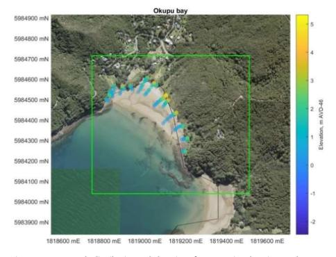
**Figure 2-7: Example distribution and elevation of survey point elevation at Okupu Bay.** Figure includes all survey points at each bay and does not delineate between beach feature types. [Aerial photograph: Auckland Council GIS, Coordinate system: NZ Transverse Mercator 2000, Vertical Datum: m AVD-46].
