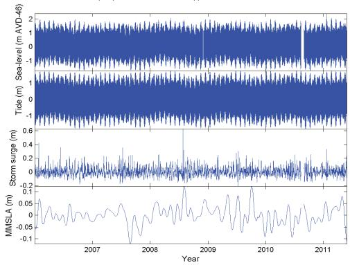
Figure 3-2: Decomposed Ports of Auckland Ltd tide-gauge sea-level record 2006–2011.
