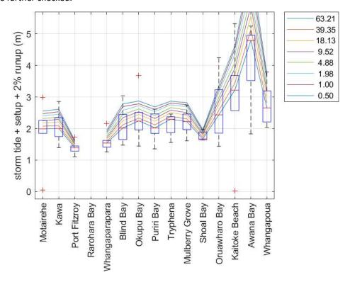
Figure 2-20: Return values of the vertical level of storm tide plus wave runup (including setup), with beach slope tuned to match the 63% AEP value against the 50th percentile value of debris line elevation.
