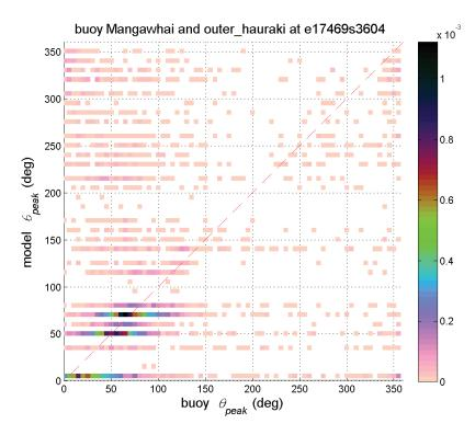
Figure 4-11: Comparison of peak wave direction (θpeak) values predicted by the outer Hauraki Gulf SWAN model with measurements from the Mangawhai wave buoy.
