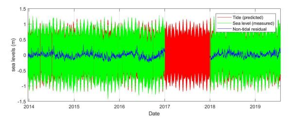
Figure 2-11: Sea level data from Great Barrier Island tsunami monitoring gauge (green), with modelled tide (red) and non-tidal residual (blue). [Raw Data: GeoNet (Station ID: GBIT), tide data: NIWA EEZ tide model]
