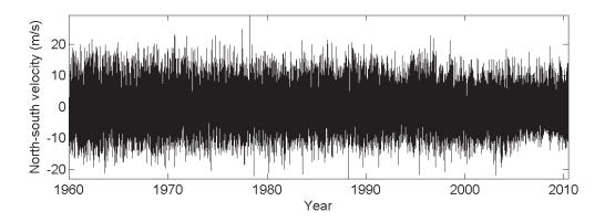
Figure 3-19: Reconstructed wind time-series used for modelling of wind-driven storm surge in the Kaipara Harbour.
