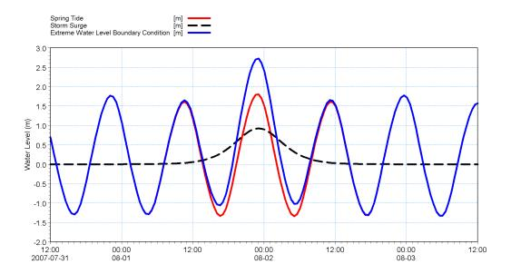
Figure 5-1 100 year ARI extreme water level open ocean boundary condition, including spring tide and storm surge components (red and black dashed lines are added together to give the solid blue line).
