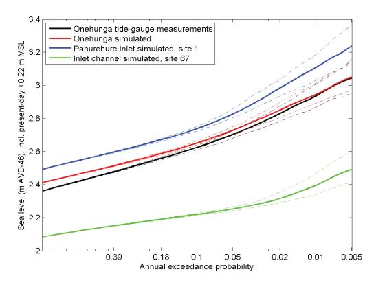
Figure 3-14: Extreme sea-level frequency–magnitude distribution at selected locations in the Manukau Harbour. (Elevations are relative to AVD-46 including +0.22 m offset for baseline mean sea level (present-day estimate). The black line is identical to that in Figure 3-13.)
