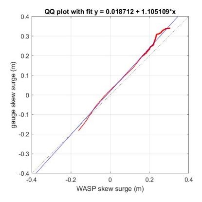
Figure 2-18: Quantile-quantile plot of skew surge values measured by the Great Barrier Island tsunami gauge, and from the WASP hindcast extracted for the same location. The red line compares corresponding quantiles from the two records, while the blue line is a linear fit to the quantile data. An equivalence line (dotted) is also shown.
