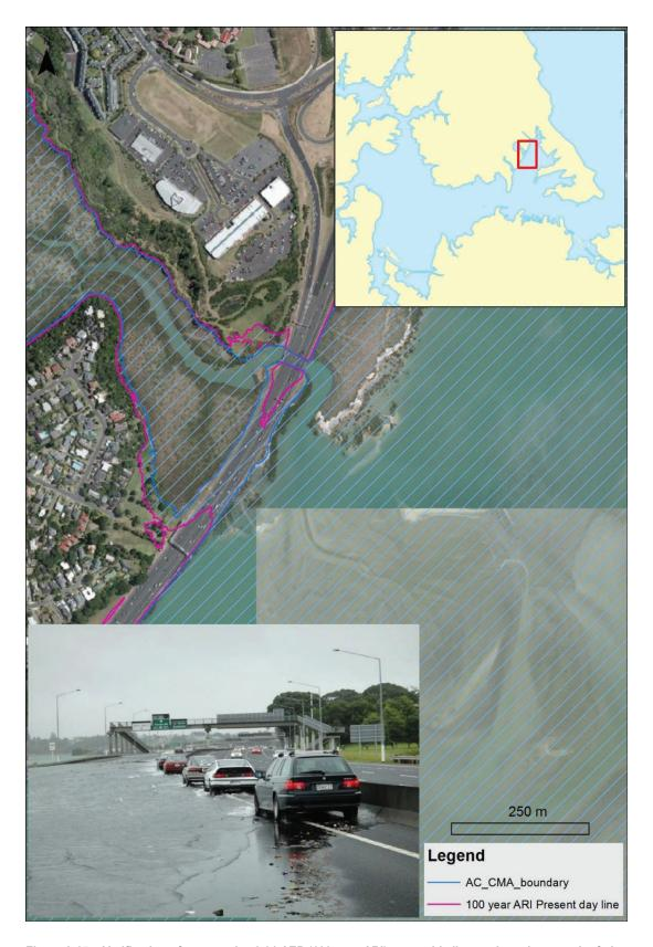
Figure 8-15: Verification of present-day 0.01 AEP (100-year ARI) storm-tide line against photograph of observed flooding on the Northern motorway during the 23 Jan 2011 storm-tide.
