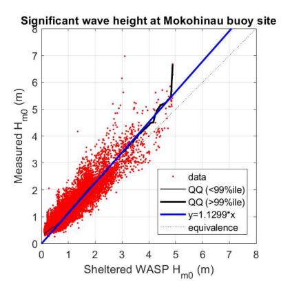
Figure B-2: Scatter plot of significant wave height at the Mokohinau buoy location derived from the WASP hindcast (with sheltering correction) against values measured by the buoy. A quantile-quantile plot is overlaid (black line), as well as a linear fit through the origin and the mean of the upper 1 percentile of the data.
