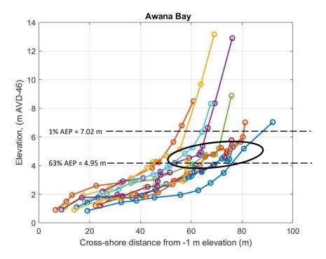
Figure 2-25: Cross-shore transects (coloured lines) measured at Awana Bay with predicted 1% AEP and 63% AEP (annotations, dashed lines) extreme storm-tide + wave runup (including setup) elevations, and identified "slope break" zone (black oval). Horizontal axis is the linear cross-shore distance from the profile interpolated to the -1 m elevation. Elevations in m AVD-46.
