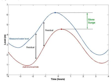
**Figure 2-19: Illustration of the definition of skew surge.** Skew surge is the difference between the maximum observed water level and the maximum predicted tidal level, which may occur at different times. [Source: <a href="https://www.surgewatch.org/definition/skew-surge/">https://www.surgewatch.org/definition/skew-surge/</a>].
