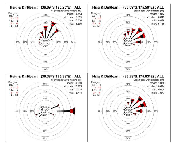
Figure 2-17: Wave roses (joint distributions of significant wave height and mean wave direction) from four WASP hindcast locations around Great Barrier Island. Output sites are NW (top left panel), NE (top right), S (bottom left) and SE (bottom right) of Great Barrier Island. Bars are oriented in the directions FROM which waves are incident.
