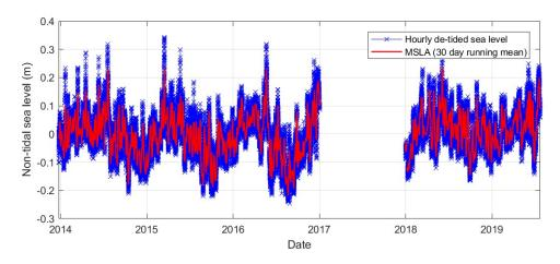
**Figure 2-13:** Non-tidal residual sea level (blue) and estimated MSLA (red). [Raw Data: GeoNet (Station ID: GBIT), tide data: NIWA EEZ tide model].
