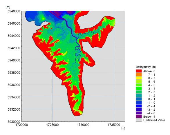
Figure 3-1 Model bathymetry and extent for southern part of Kaipara Harbour and associated floodplain. Depths are shown relative to Auckland vertical datum (1946).
