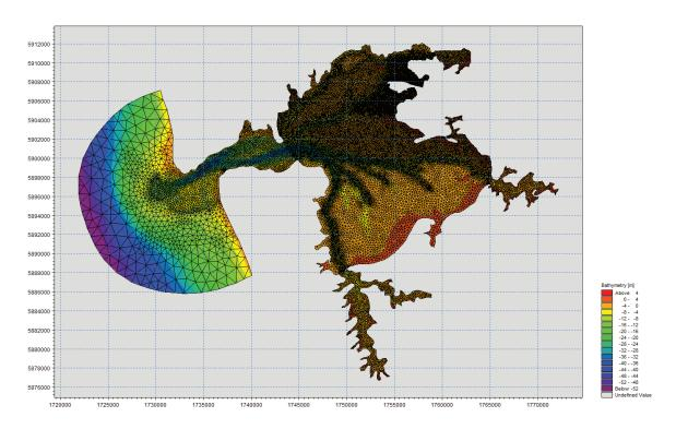
Figure 3-11: Hydrodynamic model MIKE3FM flexible mesh grid of the Manukau Harbour.
