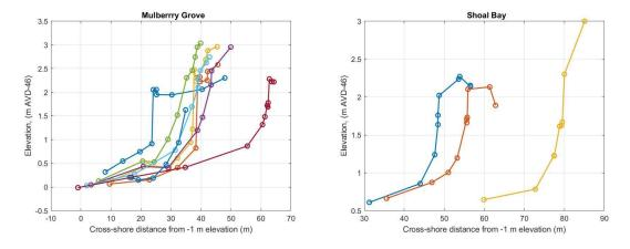
Figure 2-9: Example beach profiles at Mulberry Grove (A) and Shoal Bay (B). Horizontal axis is the linear cross-shore distance from the profile interpolated to the -1 m elevation. Elevations in m AVD-46.
