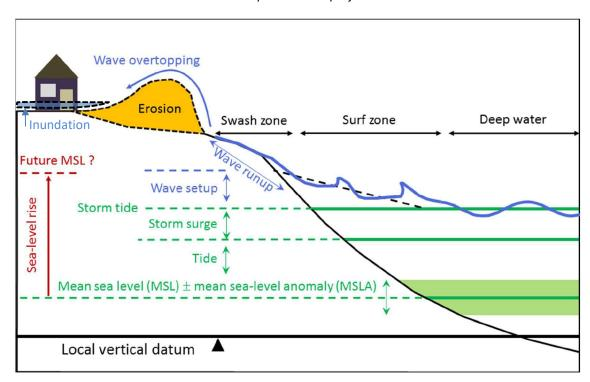
Figure 1-1: Schematic of coastal storm inundation processes. [Credit: S. Stephens (NIWA)].
