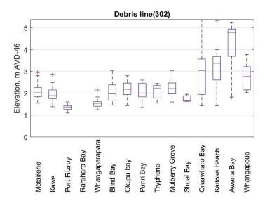
Figure 2-5: Bay by bay overview of surveyed debris features. Refer to Figure 1-3 for site location – with the last 4 sites being those on the exposed east coast. On each box, the central mark is the median, the edges of the box are the 25th and 75th percentiles, the whiskers extend  $\pm 2.7\sigma$  or 99.3 percent data coverage.
