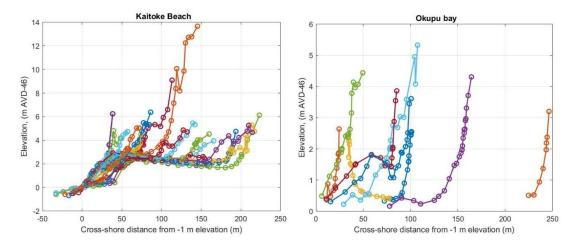
Figure 2-8: Example beach profiles at Kaitoke Beach (A) and Okupu Bay (B). See maps of survey points in Figure 2-2 (Kaitoke Beach) and Figure 2-7 (Okupu Bay). Horizontal axis is the linear cross-shore distance from the profile interpolated to the -1 m elevation. Elevations in m AVD-46.
