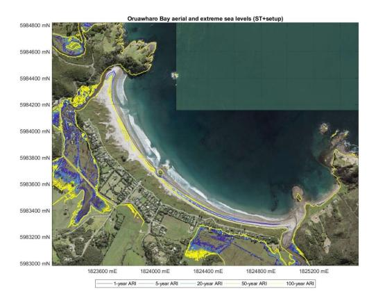
Figure 3-2: Example storm-tide plus wave setup modelling at Oruawharo Bay using static "bathtub" approach. Elevations from Table 3-1. Note that the inland areas shown to be below the model elevation are away from the coast and are subject to the limitations above streams [Aerial photograph: Auckland Council GIS, Coordinate system: NZ Transverse Mercator 2000].
