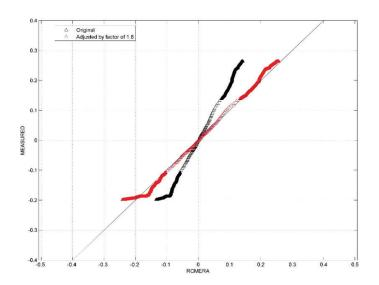
Figure 4-17: Quantile-quantile comparison of monthly mean sea-level anomaly derived from the Anawhata tide gauge and the WASP model.
