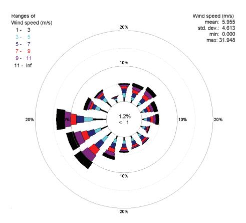
Figure 3-20: Rose plot of reconstructed wind series used for modelling of wind-driven storm surge in the Kaipara Harbour. (Wind direction relates to where wind blows from)
