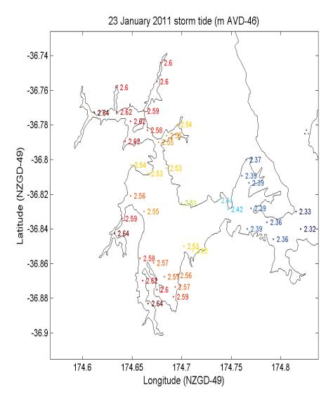
Figure 3-8: Storm-tide elevations in the Waitemata Harbour, simulated for 23 January 2011 storm-tide.
