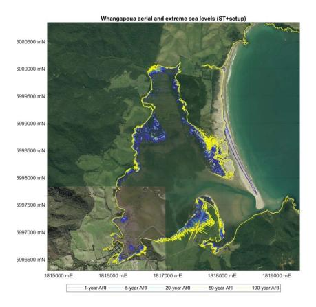
Figure 3-1: Example storm-tide plus wave setup (no runup) modelling at Whangapoua using static "bathtub" approach. Elevations from Table 3-1. [Aerial photograph: Auckland Council GIS, Coordinate system: NZ Transverse Mercator 2000].
