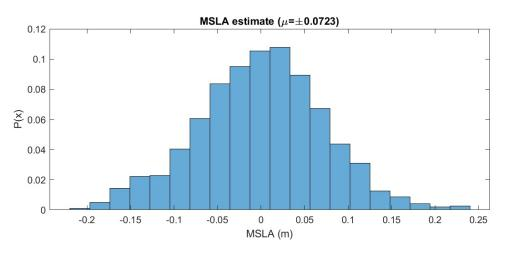
**Figure 2-14: MSLA magnitude probability distribution.** Vertical axis is probability P(x) of MSLA being observed within each MSLA (m) bin range.
