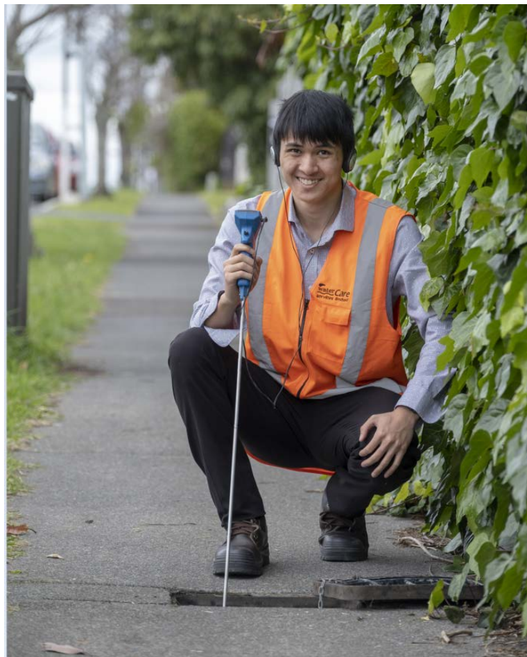
Graduate engineer Lucas Gan (right) listens to the flow of water in the pipes at Mt Wellington
