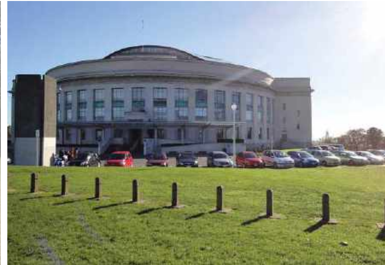
Avoid the excessive use of bollards. Consider alternative methods for restricting vehicles from pedestrian spaces.
