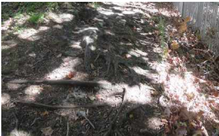
Avoid trip hazards through pedestrian routes. Raise boardwalks or elevate paths over tree roots to provide an even walking surface.
