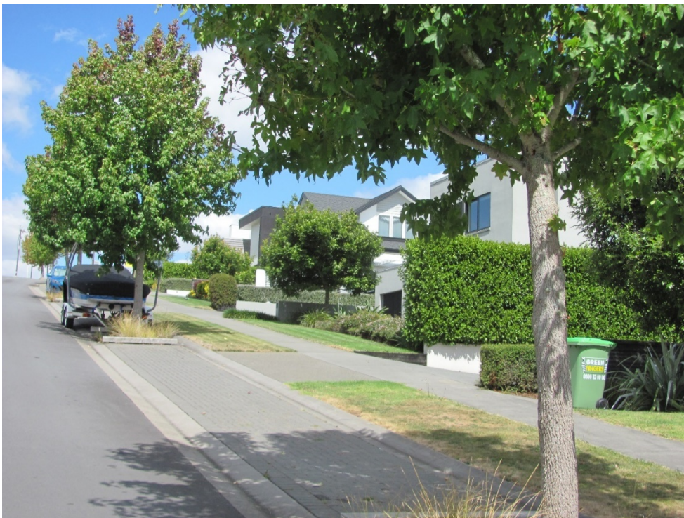
Figure 23: Example of how to address slopes through stepped horizontal components. Note the important contribution of street trees, although it would be better if the trees provided shade to the footpath not the car parks. (image from Anselmi Ridge)
