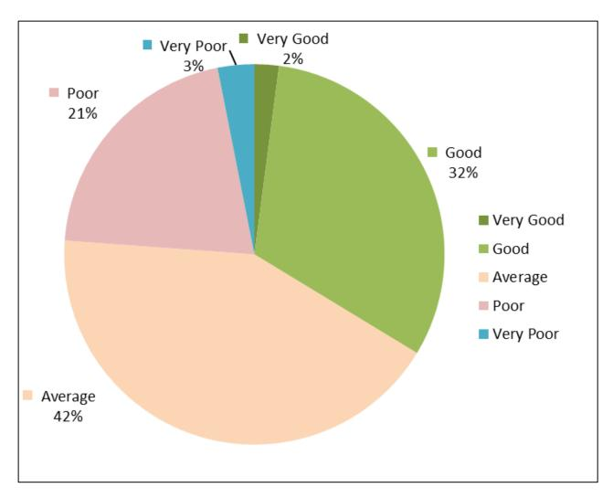
Figure 6: Oira Creek Culverts and Pipes Condition Rating (of rateable culverts/pipes).
