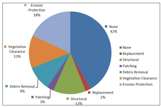
Figure 5: Oira Creek Outlets and Inlets Structures Maintenance Required Proportion (of rateable inlets/outlets).
