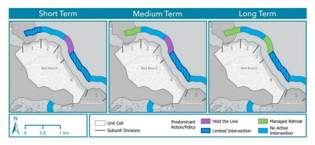
Figure 6-2: Adaptation strategies for coastal stretches within Red Beach unit area. Abbreviations: NAI (no active intervention, LI (limited intervention), HTL (hold the line), HTL-MS (hold the line, maintain structure), HTL\* (hold the line, private), MR (managed realignment).
