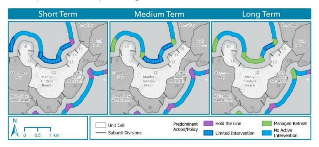
Figure 6-8: Adaptation strategies for coastal stretches within Big Manly unit area. Abbreviations: NAI (no active intervention, LI (limited intervention), HTL (hold the line), HTL-MS (hold the line, maintain structure), HTL\* (hold the line, private), MR (managed realignment).
