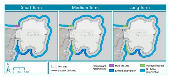
Figure 6-14: Adaptation strategies for coastal stretches within Shakespear Park unit area. Abbreviations: NAI (no active intervention, LI (limited intervention), HTL (hold the line), HTL-MS (hold the line, maintain structure), HTL\* (hold the line, private), MR (managed realignment).
