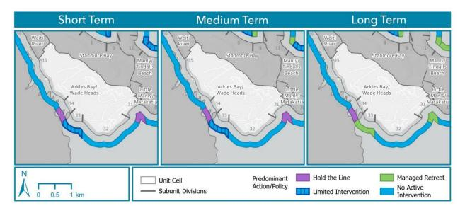
Figure 6-21: Adaptation strategies for coastal stretches within Wade Heads unit area. Abbreviations: NAI (no active intervention, LI (limited intervention), HTL (hold the line), HTL-MS (hold the line, maintain structure), HTL\* (hold the line, private), MR (managed realignment).
