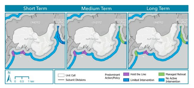
Figure 6-18: Adaptation strategies for coastal stretches within Gulf Harbour unit area. Abbreviations: NAI (no active intervention, LI (limited intervention), HTL (hold the line), HTL-MS (hold the line, maintain structure), HTL\* (hold the line, private), MR (managed realignment).
