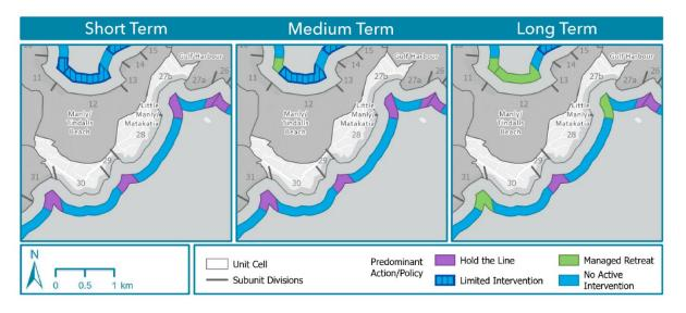
Figure 6-19: Adaptation strategies for coastal stretches within Little Manly unit area. Abbreviations: NAI (no active intervention, LI (limited intervention), HTL (hold the line), HTL-MS (hold the line, maintain structure), HTL\* (hold the line, private), MR (managed realignment).
