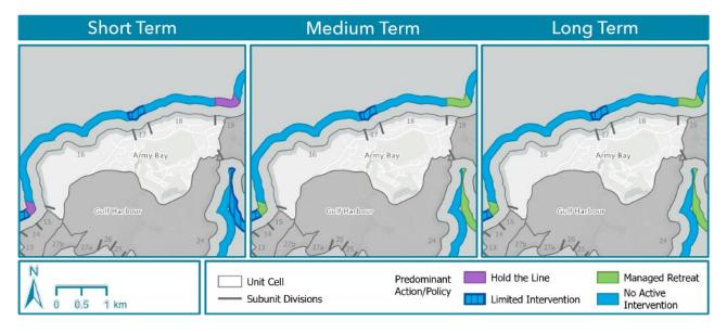
Figure 6-12: Adaptation strategies for coastal stretches within Army Bay unit area. Abbreviations: NAI (no active intervention, LI (limited intervention), HTL (hold the line), HTL-MS (hold the line, maintain structure), HTL\* (hold the line, private), MR (managed realignment).
