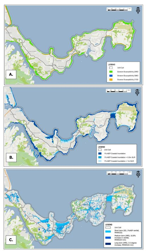
Figure 4-2: Maps showing extent of A) areas susceptible to coastal instability and erosion, B) coastal inundation, and C) rainfall flooding. AEP stands for annual exceedance probability and is the probability that a certain size flood event might occur in a single year. A 1% AEP flood is often referred to as 1-in-100-year event. SLR stands for sea level rise.
