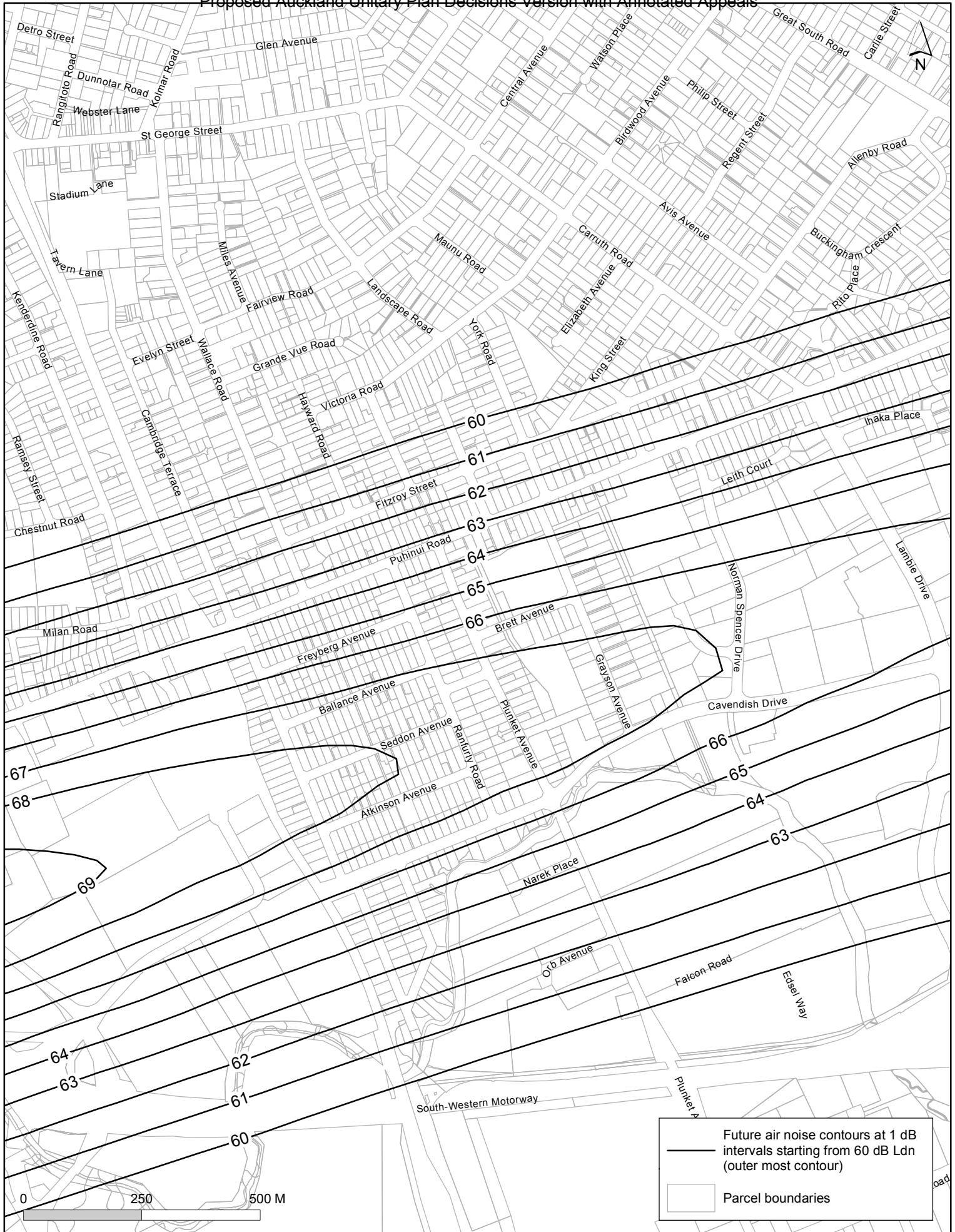
Appendix 19 - Auckland Airport Future Aircraft Noise Contours (FANC) - Aircraft Noise Overlay - Map 6
