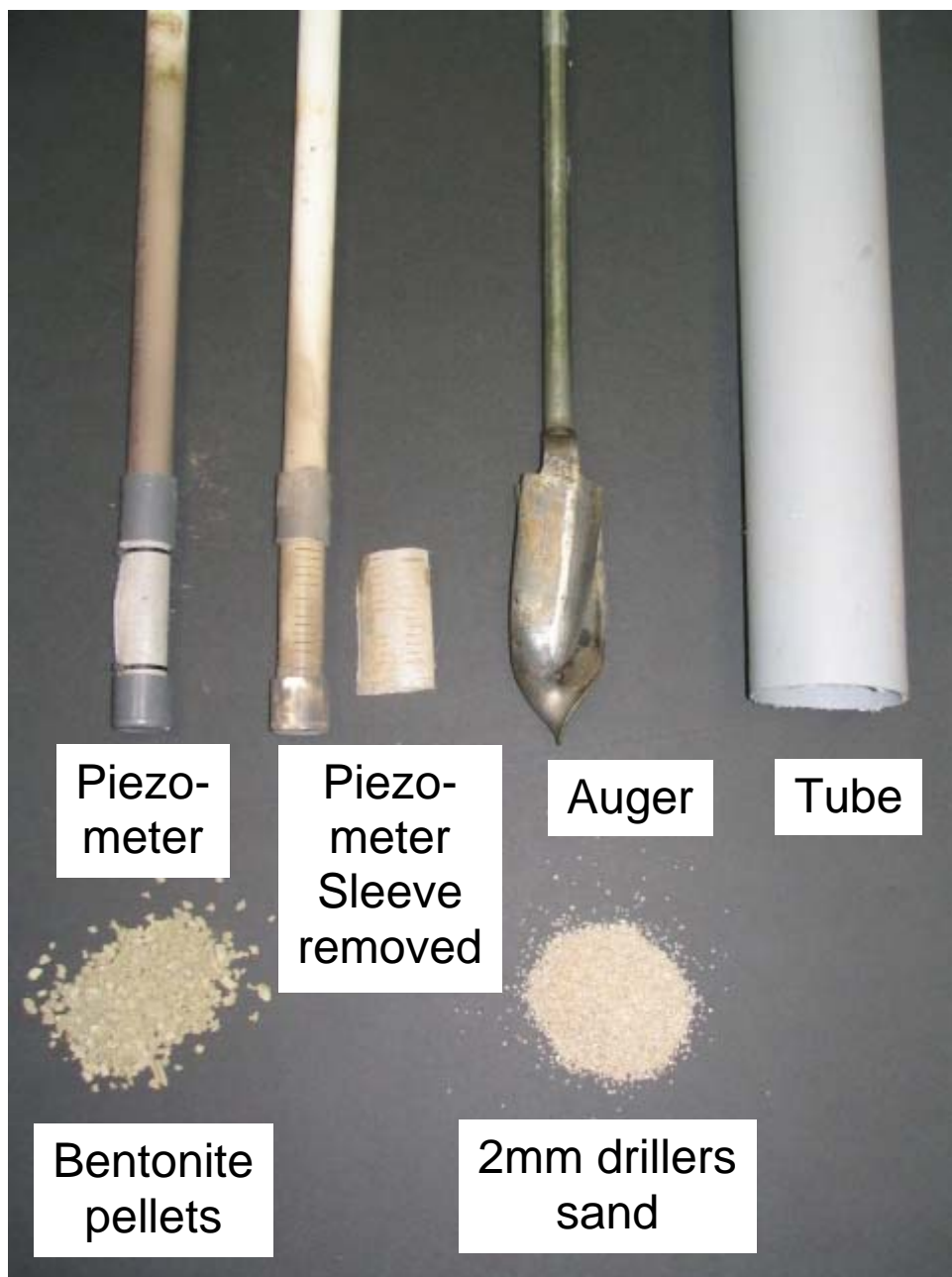
Figure 4: Piezometer installation gear.
