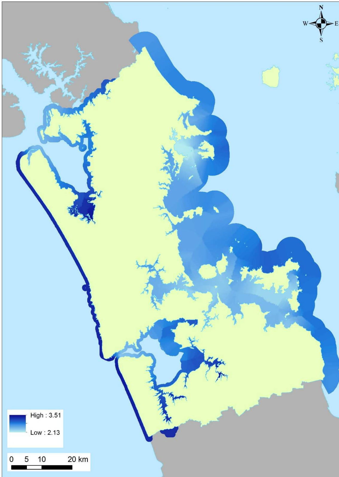
Figure 8-6: Map of Auckland region with water surface for 0.01 AEP (100-year ARI) elevations.
