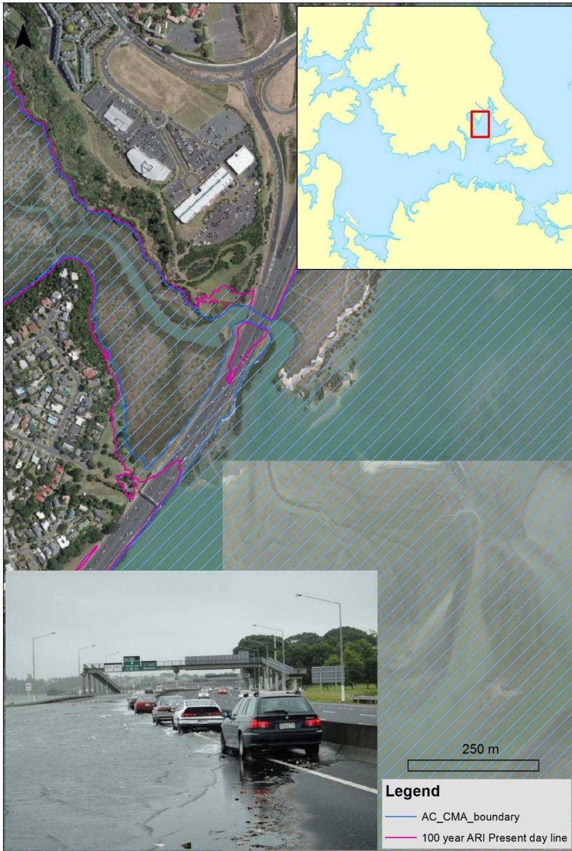
Figure 8-15: Verification of present-day 0.01 AEP (100-year ARI) storm-tide line against photograph of observed flooding on the Northern motorway during the 23 Jan 2011 storm-tide.
