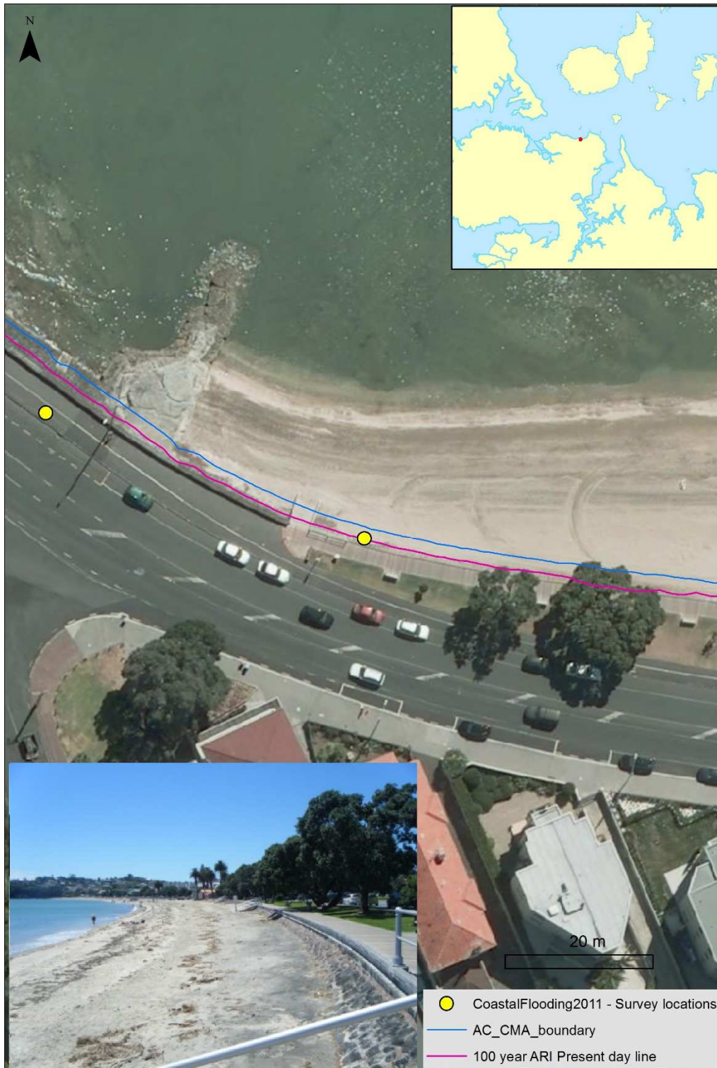
Figure 8-11: Verification of present-day 0.01 AEP (100-year ARI) storm-tide line against surveyed location of maximum flood incursion during 23 Jan 2011 storm-tide, at Saint Heliers Bay. Pink line marks modelled 0.01 AEP storm-tide line. Blue line marks coastal marine area (CMA) boundary.
