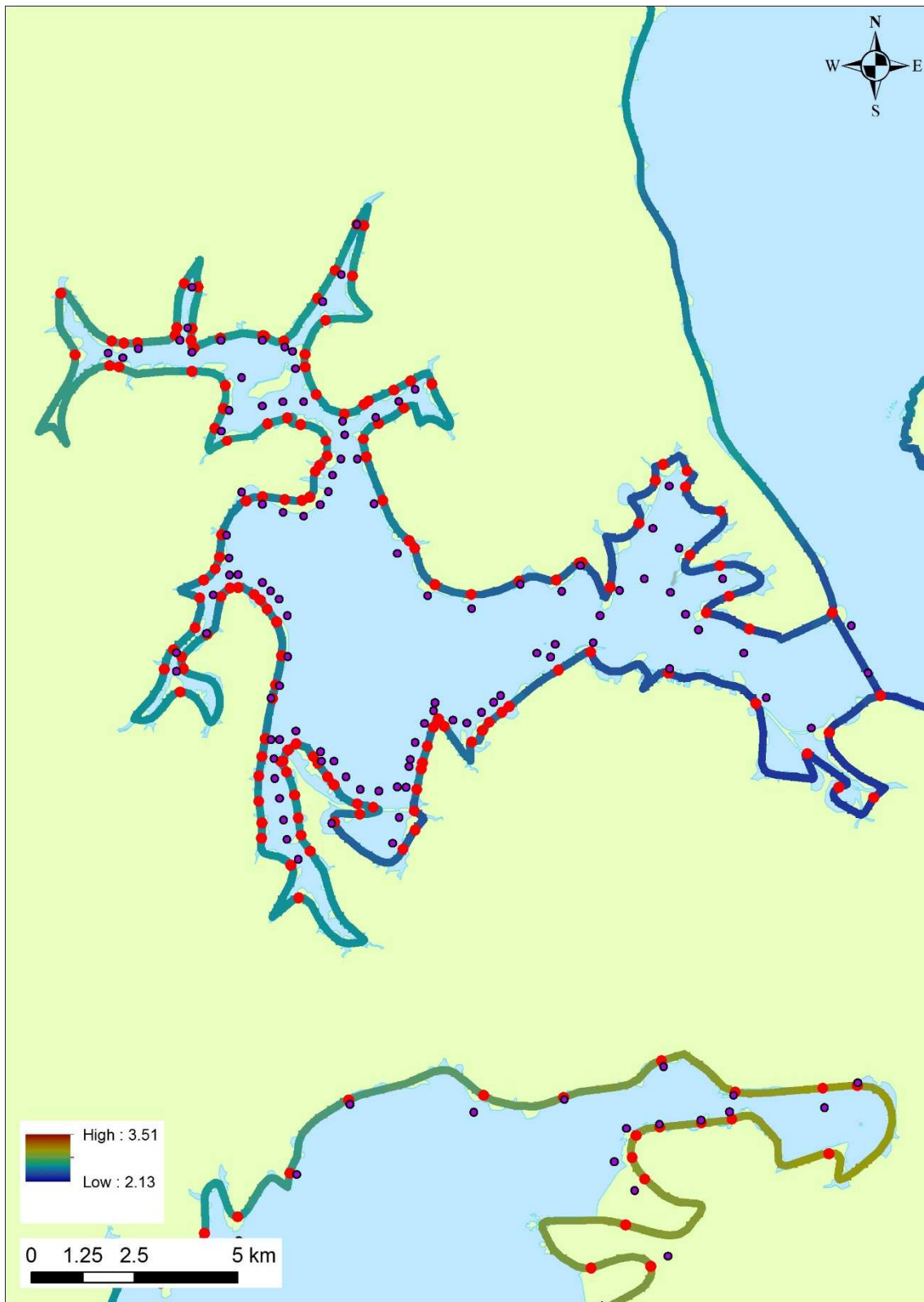
Figure 8-3: Map of Waitemata Harbour with interpolated elevation values on the simplified coastline. “Hot points” along the coastline are marked in red, modelled sea-level output locations in purple.
