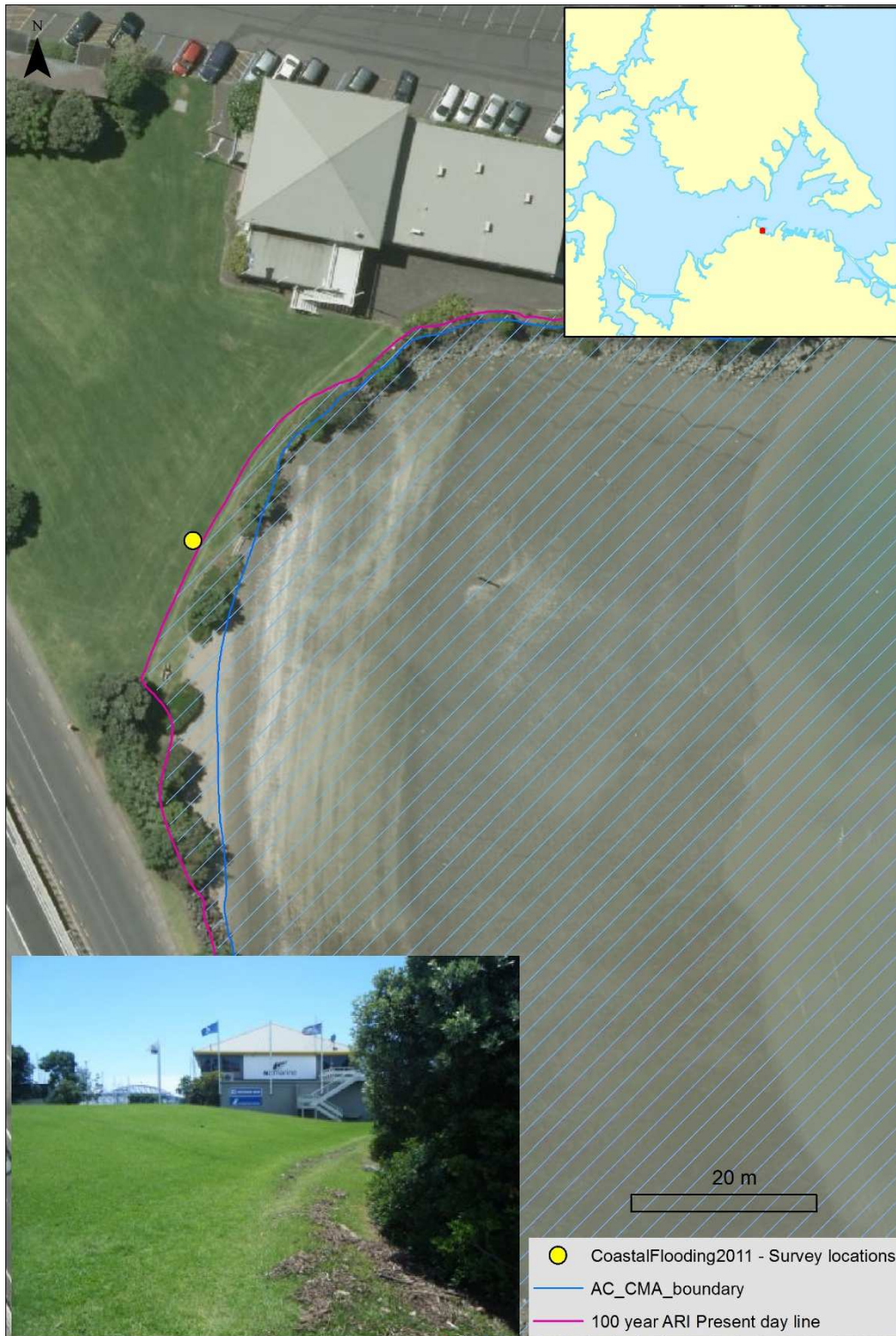
Figure 8-13: Verification of present-day 0.01 AEP (100-year ARI) storm-tide line against surveyed location of maximum flood incursion during 23 Jan 2011 storm-tide, at Saint Marys Bay. Pink line marks modelled 0.01 AEP storm-tide line. Blue line marks coastal marine area (CMA) boundary.
