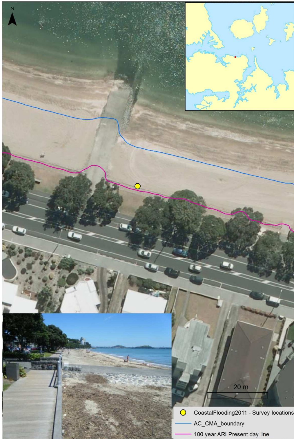
Figure 8-9: Verification of present-day 0.01 AEP (100-year ARI) storm-tide line against surveyed location of maximum flood incursion during 23 Jan 2011 storm-tide, at Kohimarama. Pink line marks modelled 0.01 AEP storm-tide line. Blue line marks coastal marine area (CMA) boundary.
