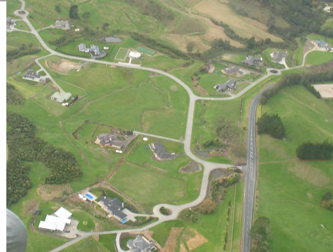
Figure 25. New driveways with a maximum grade of more than 1:8 or accessing more than 4 dwellings are required to be constructed in concrete
