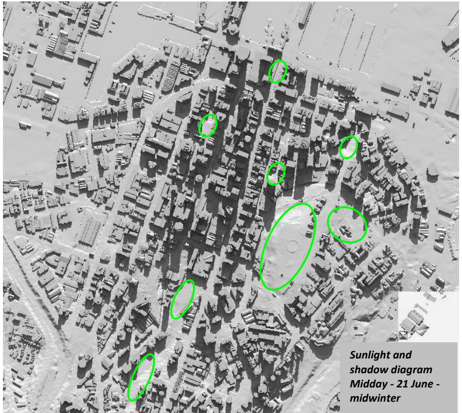
The admission of sunlight to public places control influences building height. The top image shows the extent of that influence for Albert Park and Old Government House with lower buildings. The shadow diagram below shows the location of public places with sunlight protection and how successful the approach has been ensuring midday sunlight in mid winter.
