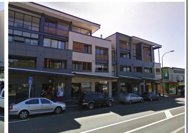
4. New and larger buildings that line the main street are often broken up with a vertical emphasis so they don't stand out against the neighboring slimmer heritage buildings. The façade of this building has been broken up with colour and by using negative details.
