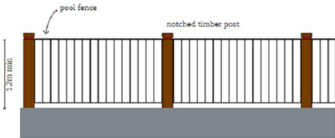
Figure 14 - Fencing Detail 4 - Green Infrastructure Zone
