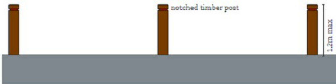
Figure 13 - Fencing Detail 3 - Public Open Space - Conservation
