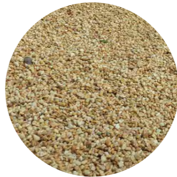
Hoggins (Compacted Aggregate + Lime)
